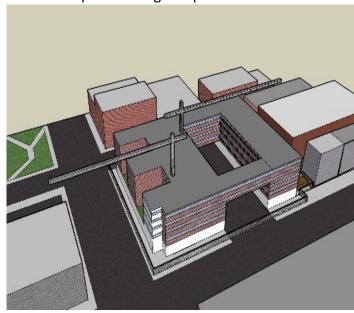
remove the cranes and pour more concrete to finish the slabs. If both cranes were located on Festival Street, then all concrete work would be done all at once and they would not have to deal with filling the wholes later.
